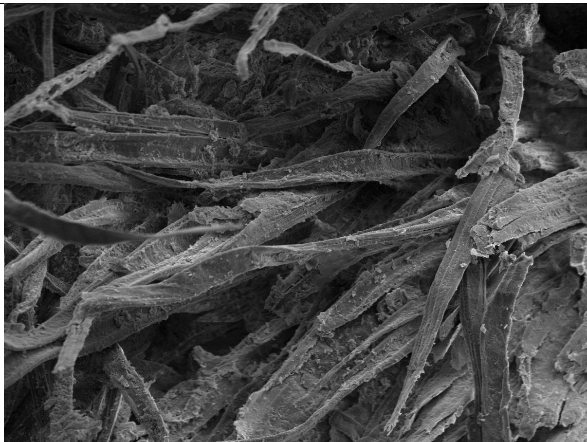
Figure 5. Detail of K546-5 showing fibrous material embedded in substrate.
