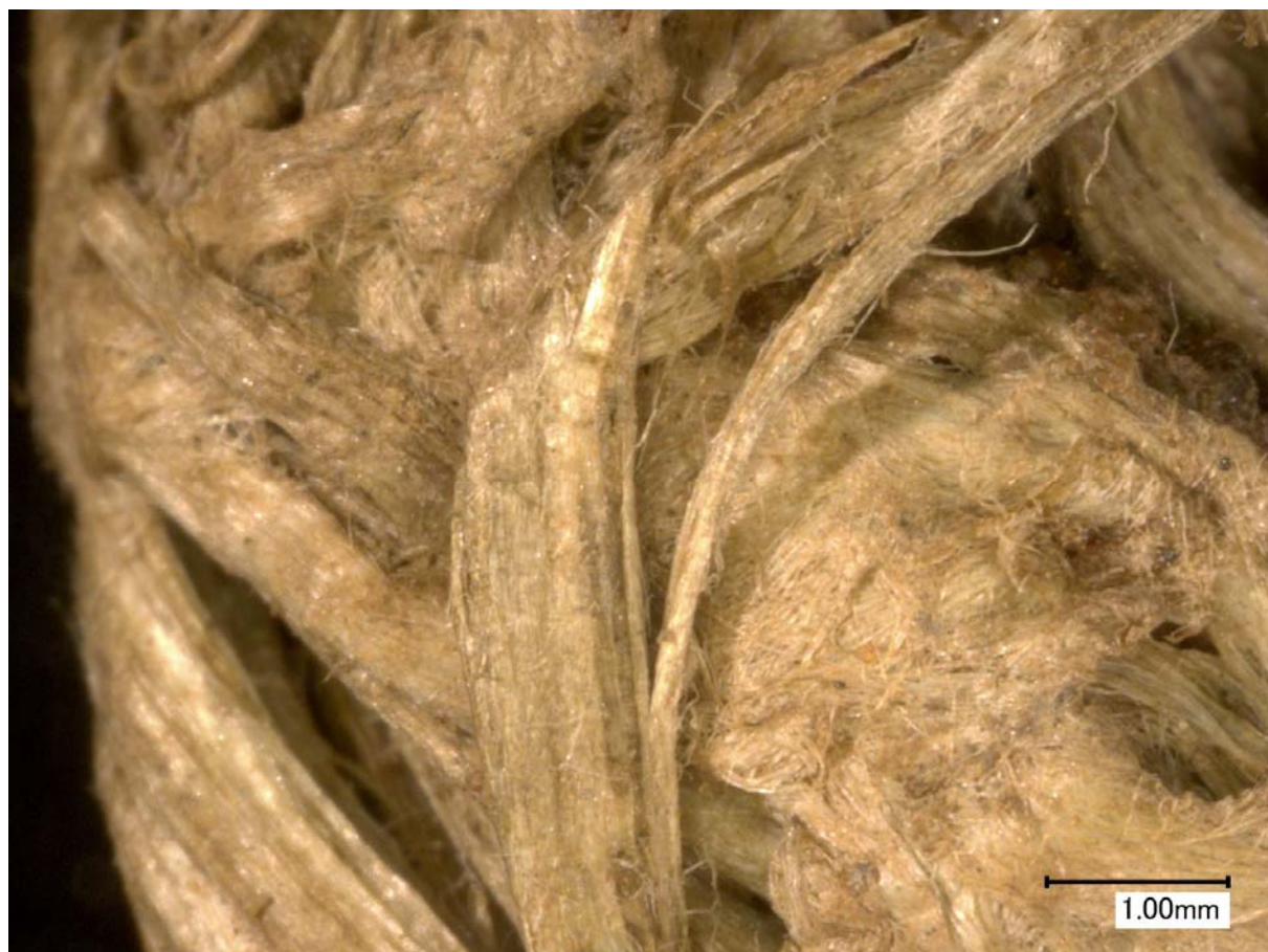
Figure 2. Detail of K787-1 sample collection point showing embedded nature of fibrous material.
