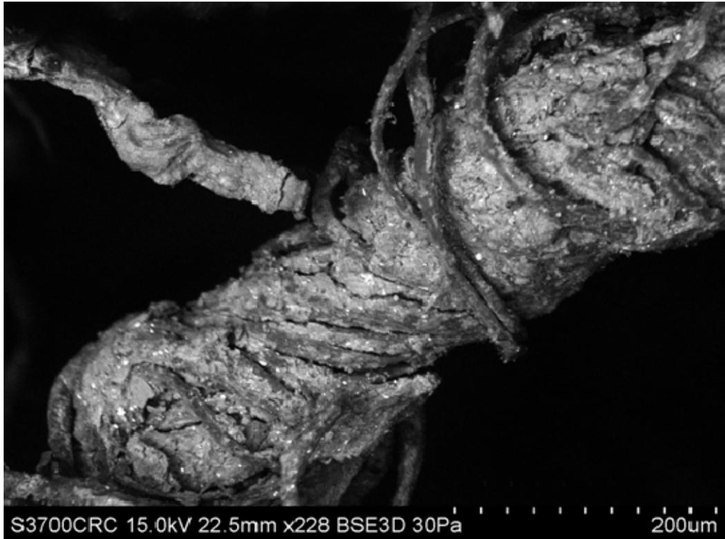
Figure 16 BSE image of main textile fragment K281c where yarn twist is masked
