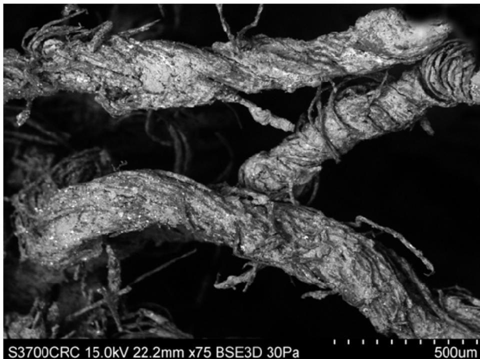
Figure 18 BSE image of main textile fragment K281c where yarn twist is masked
