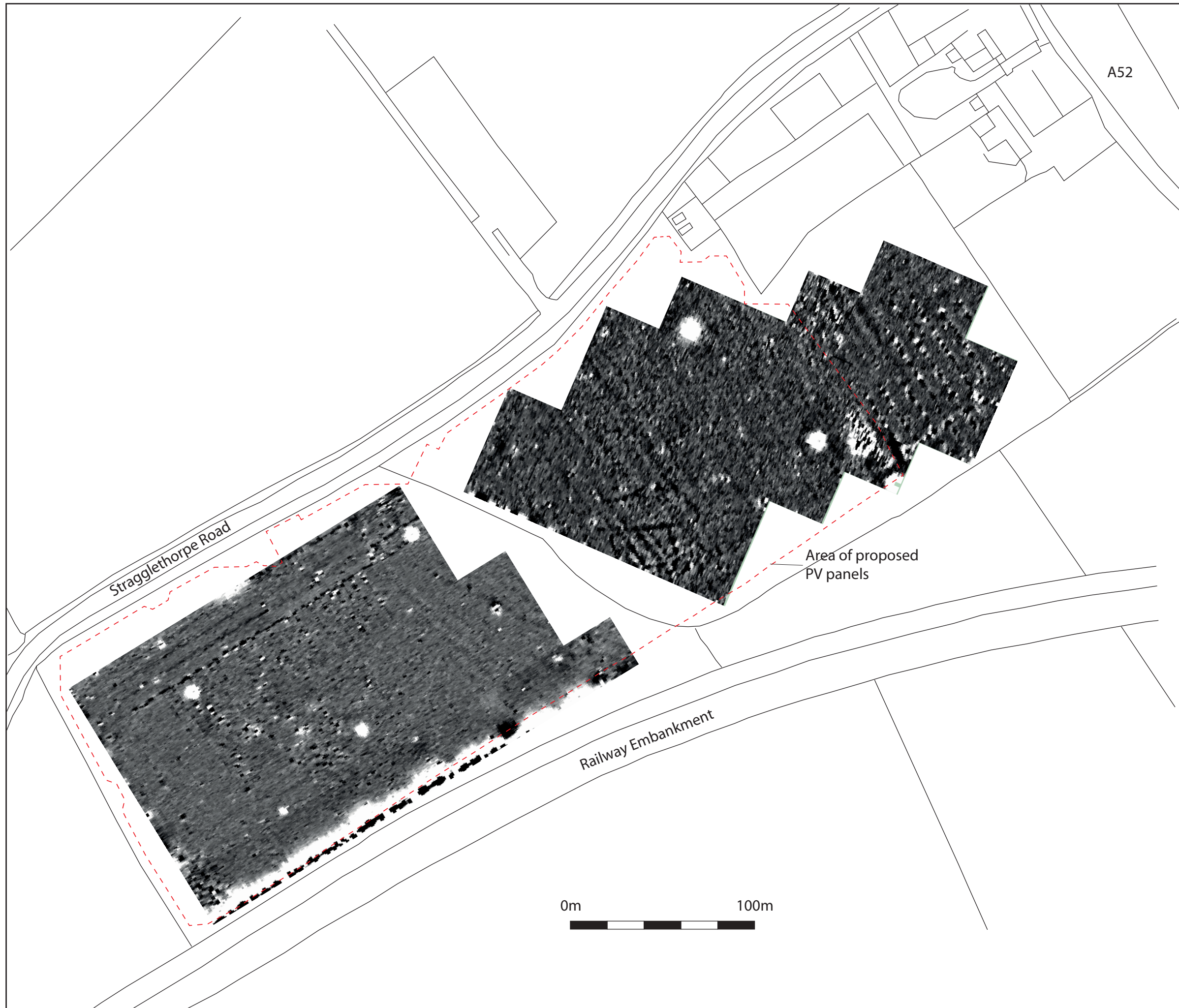
Figure 5: Geophysical survey results overlaid on Ordnance Survey data.
