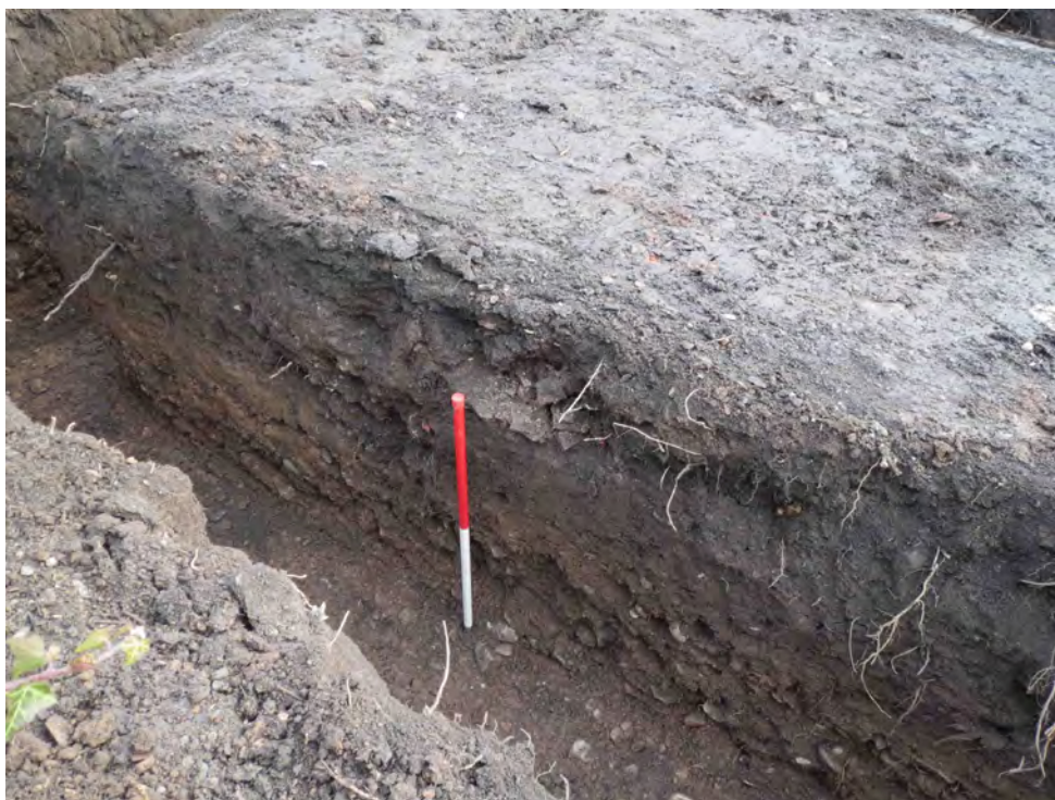
Plate 22. Oblique view of Section D (Footing 2), showing the general soil sequence comprising topsoil (100), subsoil (101) and natural (102). Looking east-southeast.
