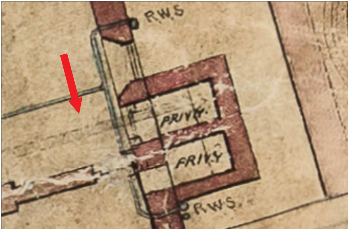
Plate 39: Extract from 1855 plan indicating the 'earth pipe' entering the privy tower below the mill floor
