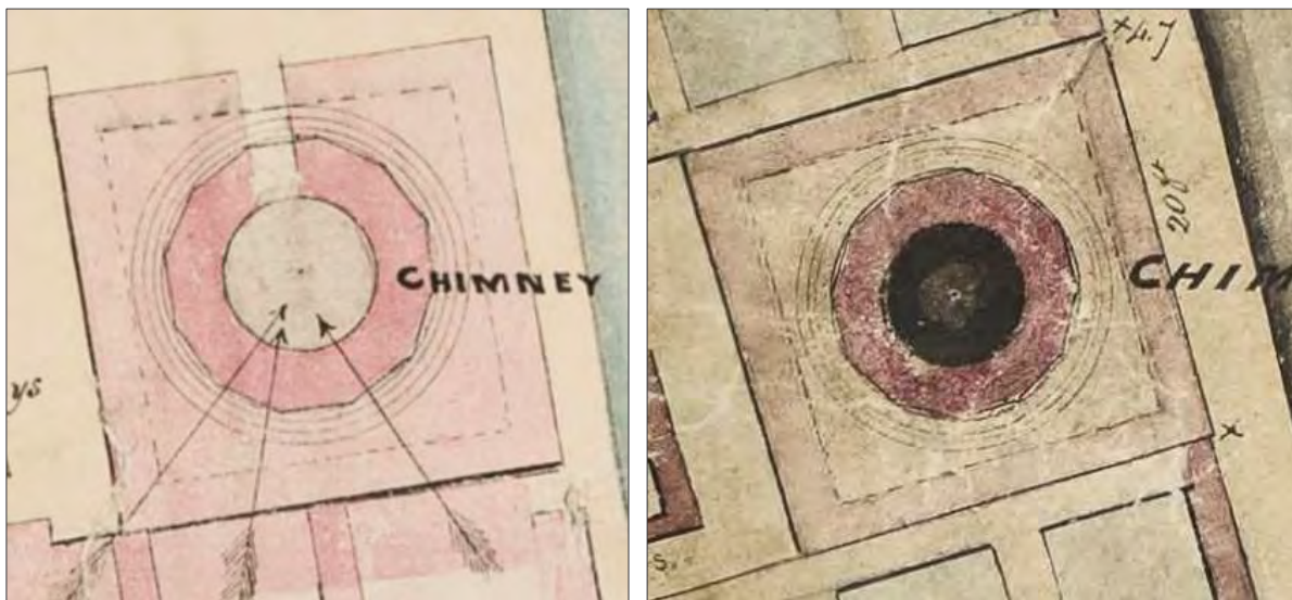
Plate 36: Extracts from the 1849 and 1855 plans showing the cross section of the chimney base
