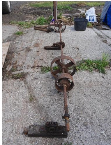
Figure 14: Cast Iron Drive Shaft.
