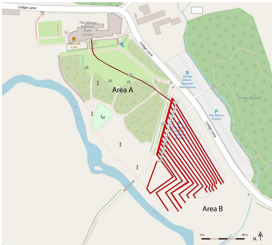
Figure 4: Site plan with the location of the trenches required for the ground source heat pump indicated in red.
