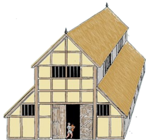
30: building F4 if posts supported the aisle of a timber-framed structure (Millum 2017)
