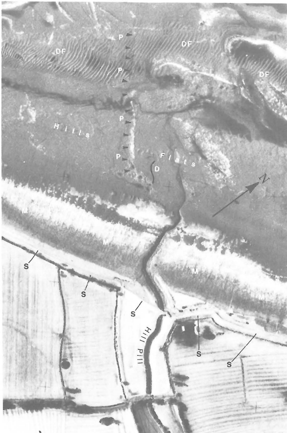
Figure 11. Air photograph (area 525-800m) showing the intertidal zone and immediate alluvial hinterland in the vicinity of the mouth of Hill Pill. D - drain bottom; DF - field of gravel dunes; M - active salt marsh; P - arrowed line of palaeochannel; S - seabank.
