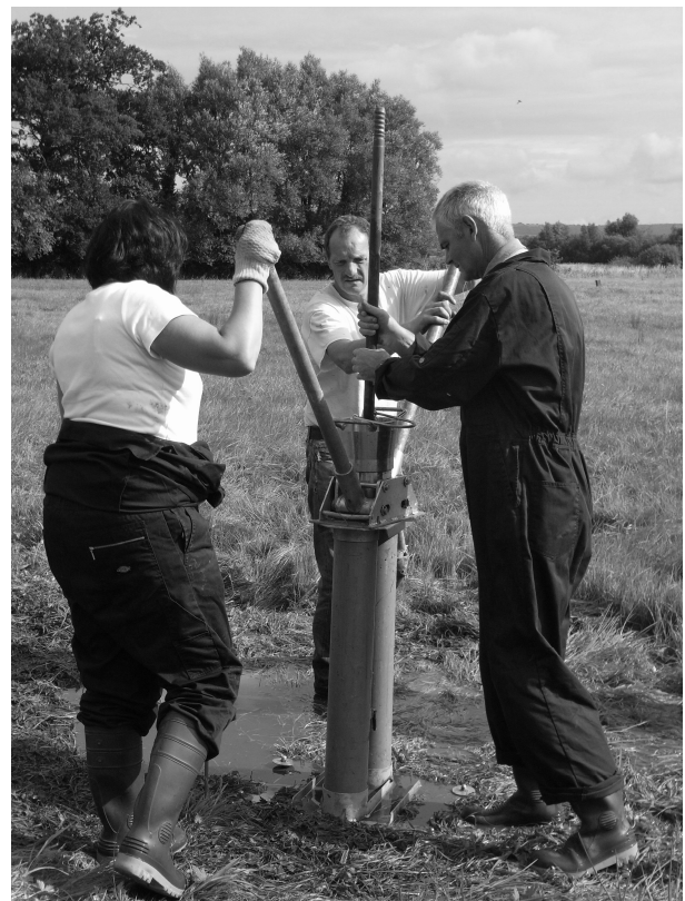
Figure 8. Installing the TDR access tubes at Glastonbury Lake Village.
