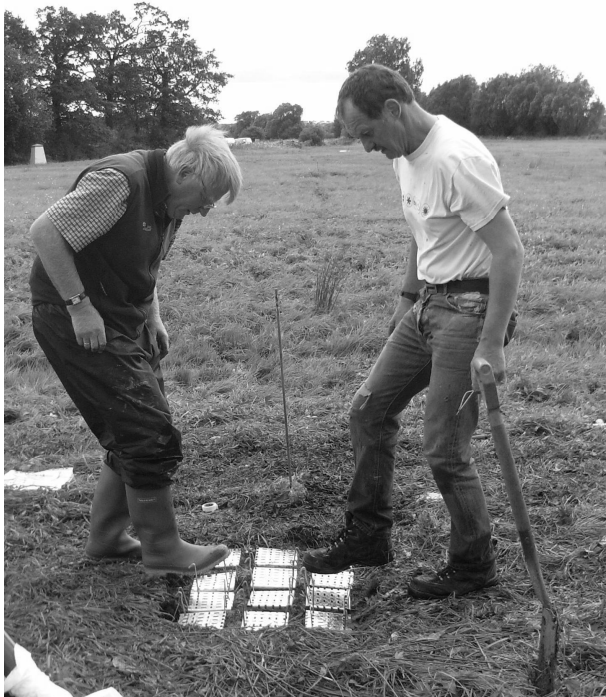
Figure 7. Installing protective metal plates over the monitoring equipment at Glastonbury Lake Village.
