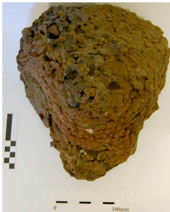
Figure 14. Slag block from furnace 28 (89), viewed from above. Scale 0.1 m.
