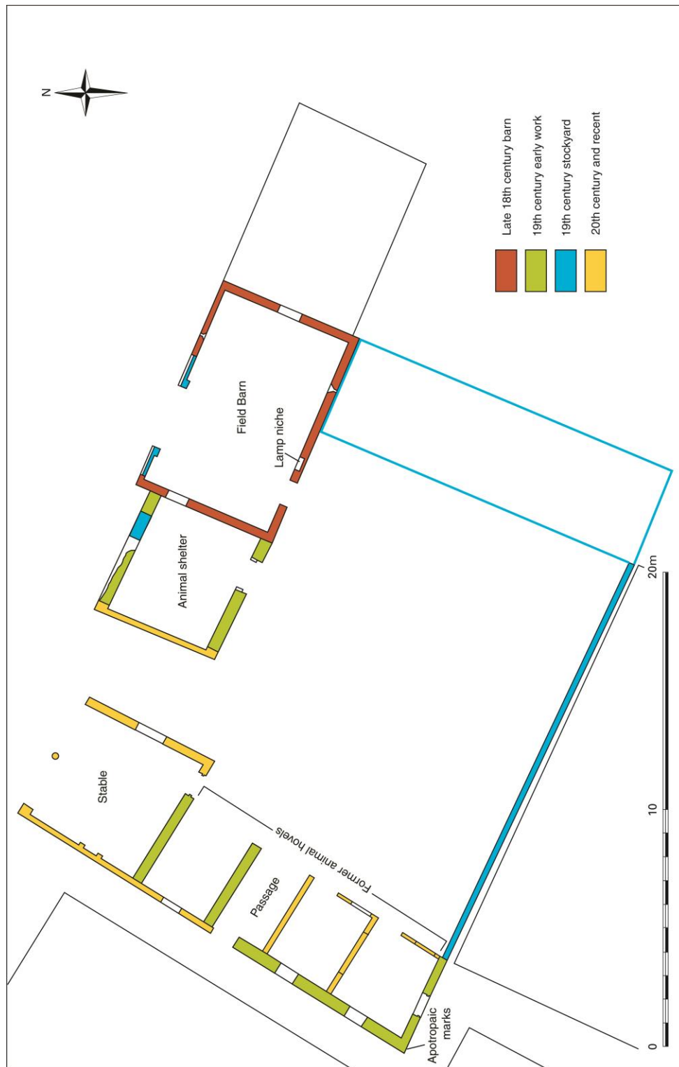
Fig 3: Plan of the farm buildings phased (Andy Isham after Roger Coy Partnership).
