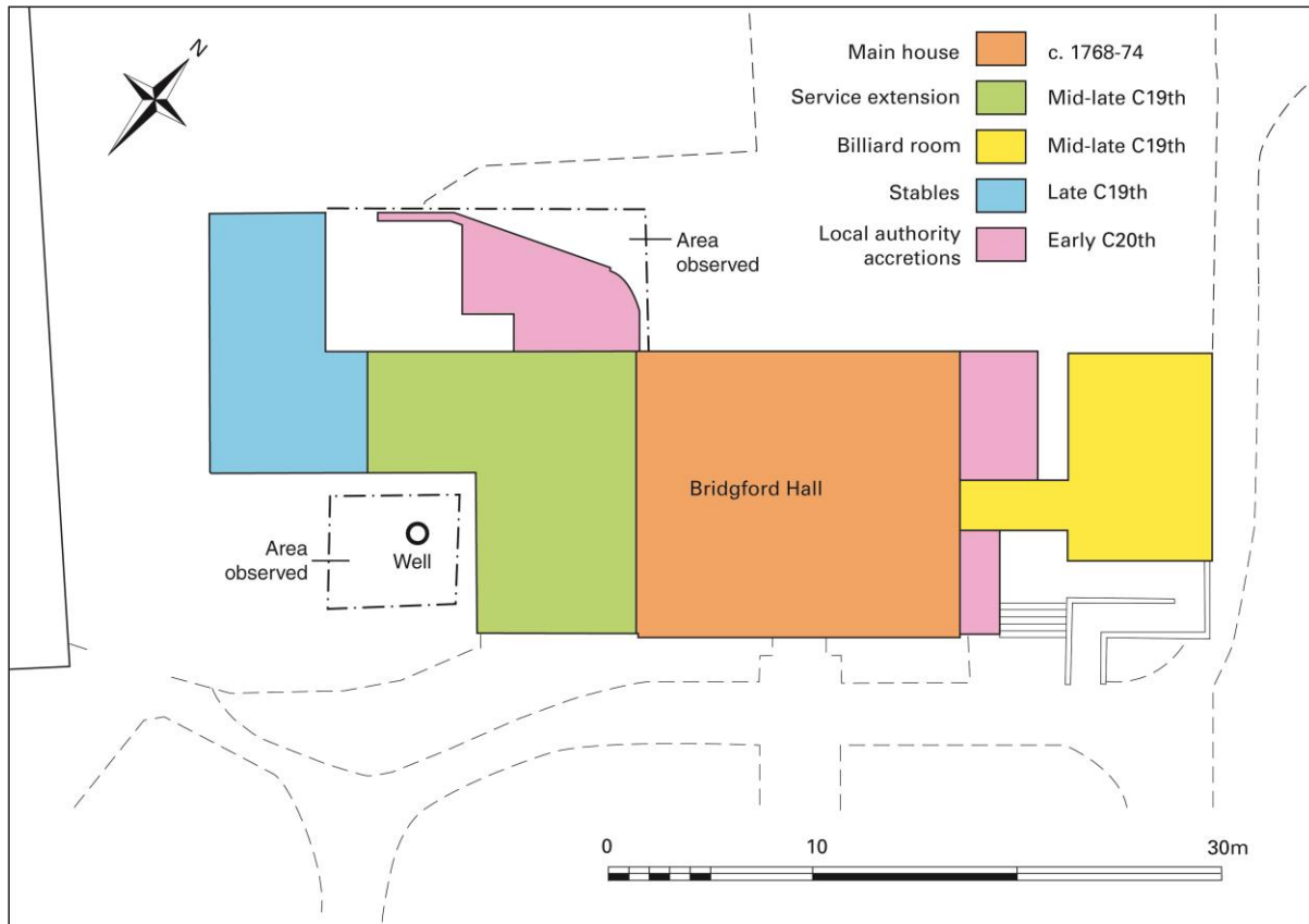
Fig 2: Block-phasing of the hall, with areas of archaeological monitoring (Andy Isham, with acknowledgement to Purcell, Architects).
