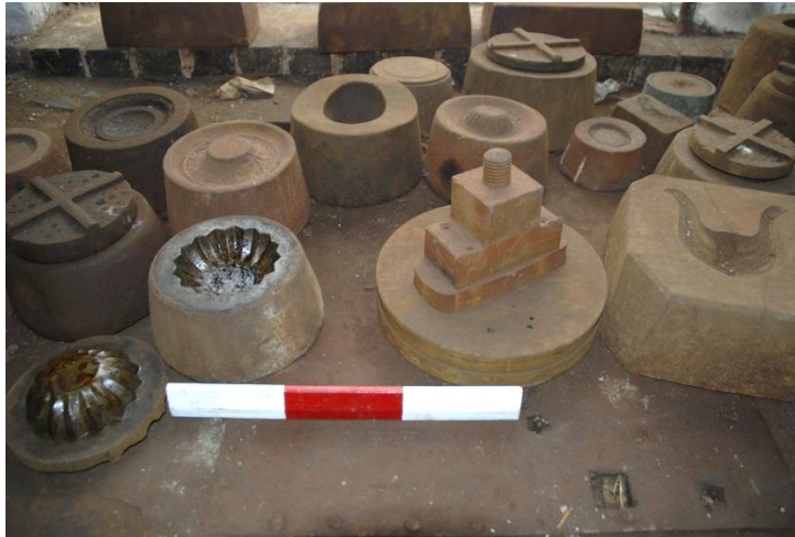
Fig 41: Stamps and dies stored on benches in EG31, a frontage window onto Vittoria Street behind. The stamp to the far right is one half of a pair of tea-pot spouts. The gouges in the bench-top at bottom right show that in a former room-use fly-presses were formerly located here; scale 30cm.
