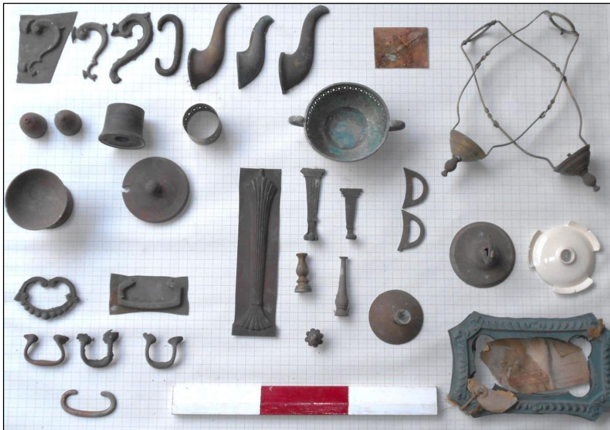
Fig 113: Finished and part-finished cast or stamped artefacts found in profusion around the ground and first floor of Unity Works (principally EG 49 and 51 and EF34): handles, spouts, salt and pepper pots (pattern as described in report above), matching mustard pot, bowls, lids, knops, stems, feet, light fittings, regimental badge (The Parachute Regiment); scale 30cm and photographed against 1cm graph-paper background.
