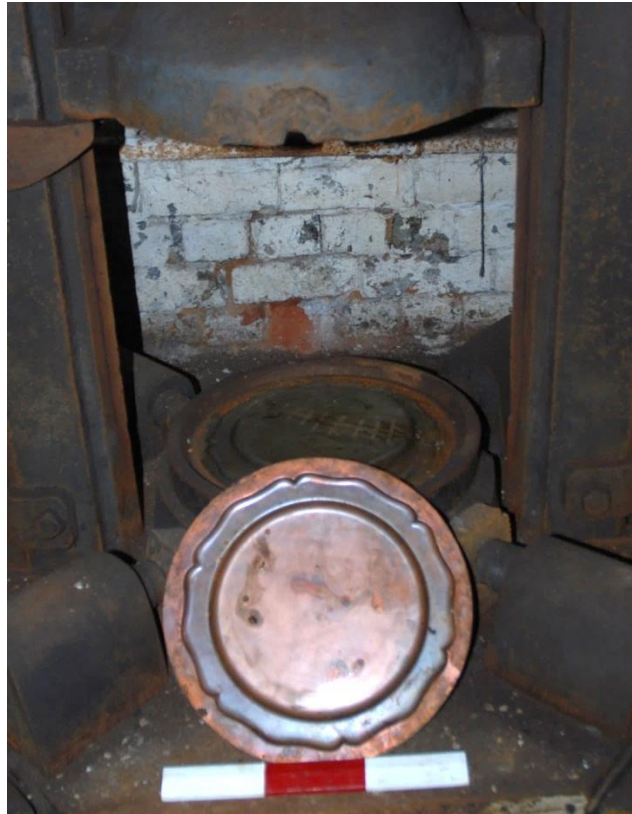
Fig 16: The 10" copper or nickel silver tray and its die stamp, still set for production; scale 30cm
