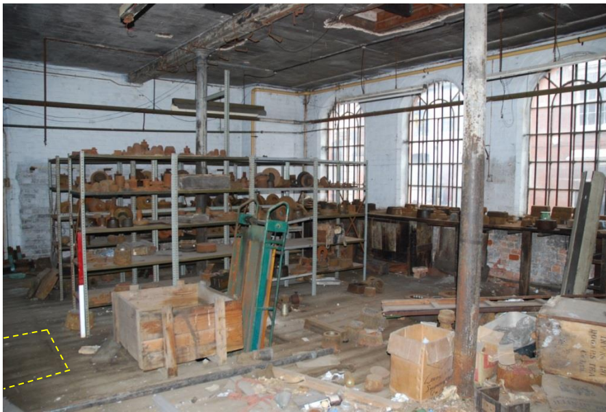
Fig 38: Room EG31, looking North-east. Note the covered-in ceiling. Both the bench and the shelves are full of stamps and dies. The turquoise coloured cellar hoist through an open floor-hatch can also be seen from below in Fig 28 (above). Another closed hatch is marked in yellow. Scale 1m.
