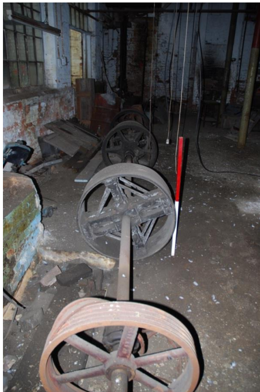
Fig 52: A former drive shaft and drive wheel, ex situ ; scale 1m. The drive wheels are in laminated wood to prevent the belts slipping. Secondary, iron wheels were often grooved for rubber belts (that in the foreground for four) or flanged to prevent slack or angled belts from sliding off.
