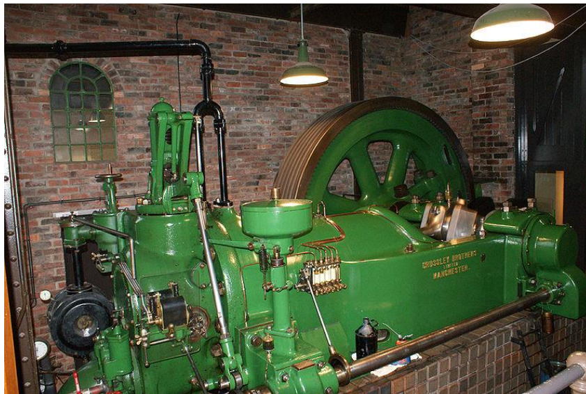
Fig 71: A typical (large) Crossley Gas Engine (Kelham Island Industrial Museum) - pre-First World War
