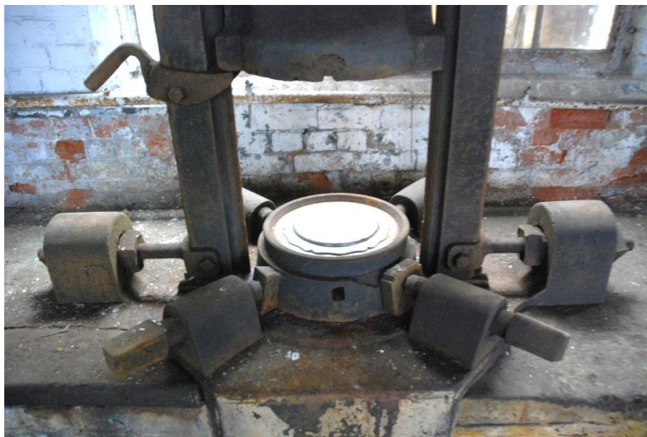
Fig 50: The biggest surviving press with stamp for a hollow-ware 10" plate or tray, held in place by a ring of four inclined bolts, called 'poppets'. Note the polygonal shock-absorbing iron 'anvil' within the brick and timber-topped bench. This prevented the bricks in the bench from shattering under repeated impacts. Note the manual brake lever on the left
