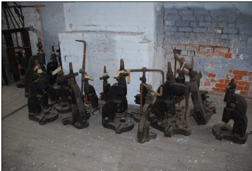
Fig 61: ES29 – a collection of dismantled fly-presses of different types and sizes, such as the Denbigh or the Norton no1, no 38 and no 58, mostly by Sweeney and Blocksidge, Saltley, Birmingham, but some by Hazelwood and Dent, Birmingham. The latter company was established in 1885, but its premises were severely damaged by fire in 1928.
