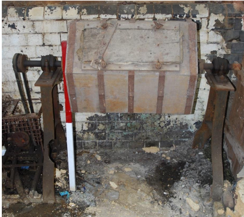
Fig 76: belt-driven tumbler drum for polishing, so called 'barrelling', discarded in the covered yard; note the belt and drive low down to the left; scale 1m
