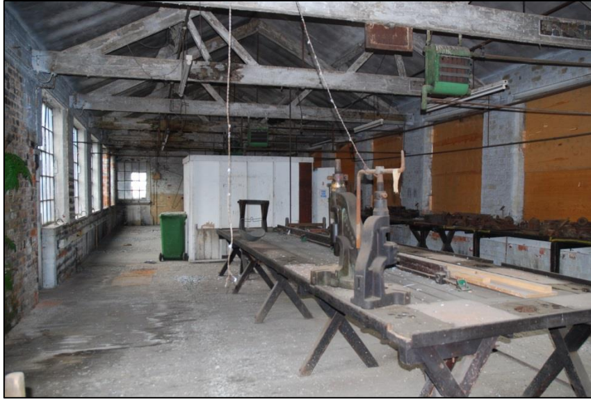
Fig 60: ES29 west end looking east to the stair. The centre benches all have fly-press fixing holes. All work-stations along the walls and the centre benches were provided with electricity and a fixing for an angle-poise lamp, style icon of the 1940s and uniform at a date when war work meant national investment at the end of a decade of economic depression.
