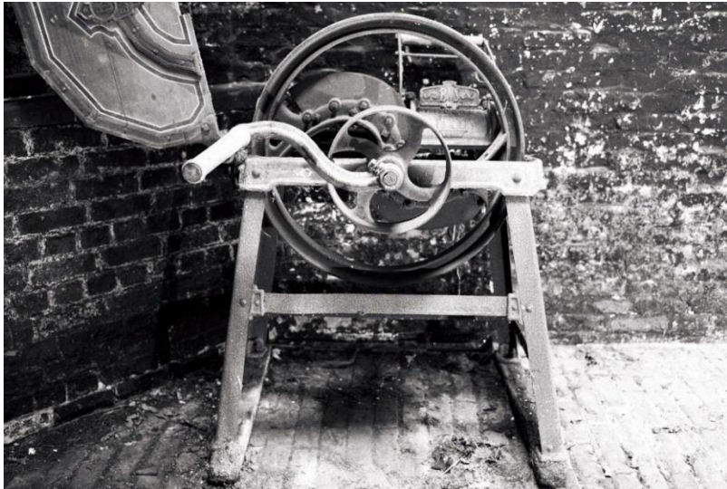
Fig 33: The chaff cutter; guard up.
