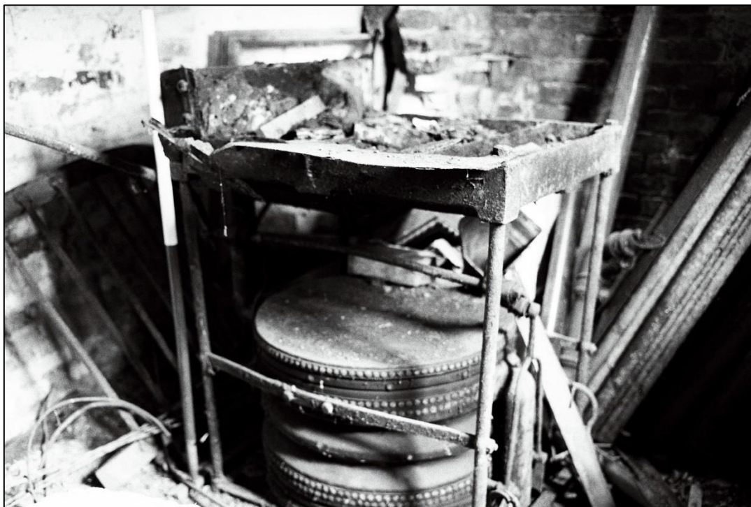
Fig 40: The heart of the forge – an excessively heavy mobile bellows and hearth combined; scale 1m
