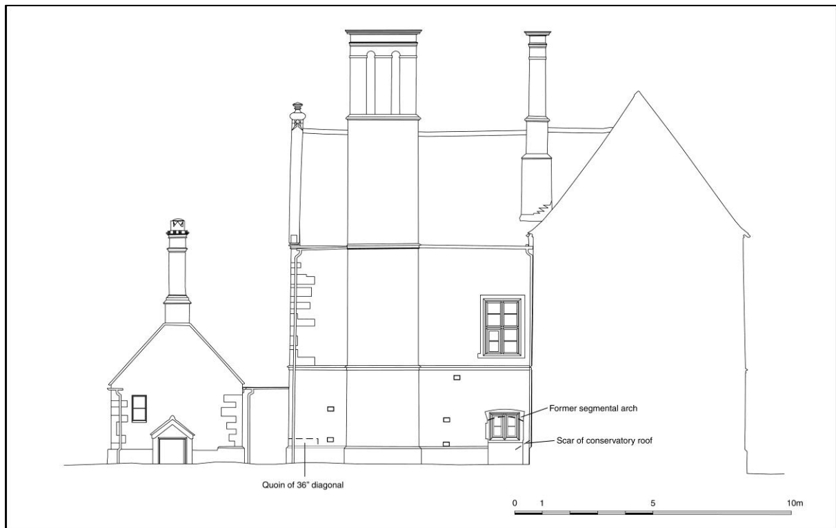
Fig 32: Drawing of east elevation of the south range showing alterations (Andy Isham).
