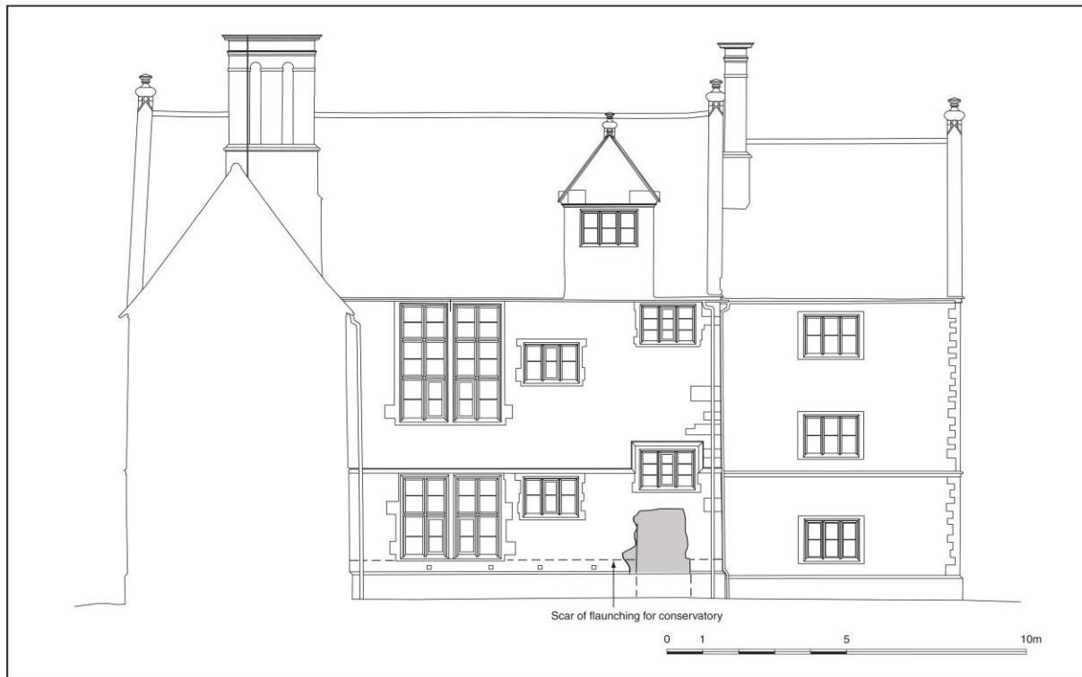
Fig 30: South elevation drawing showing alterations (Andy Isham)
