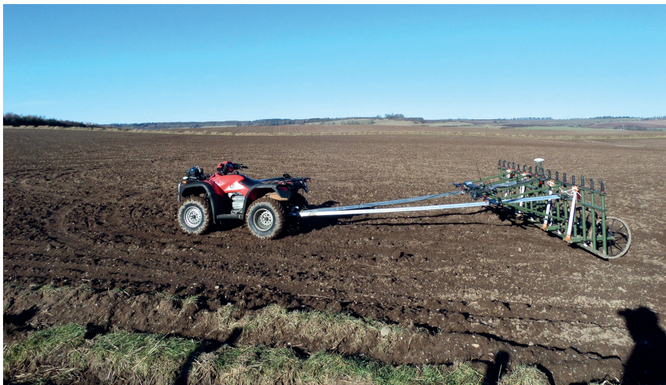
Figure 2.26 SENSYS Magneto MX V3 used in the large-area survey in February 2015 (photo: G Konieczek, SENSYS GmbH)
