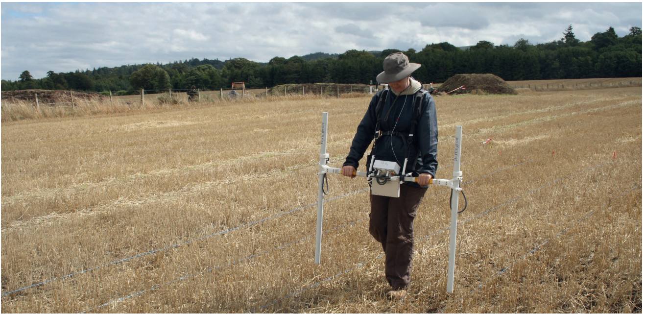
Figure 2.22 Gradiometry survey in 2010: Bartington Grad 601 in use
