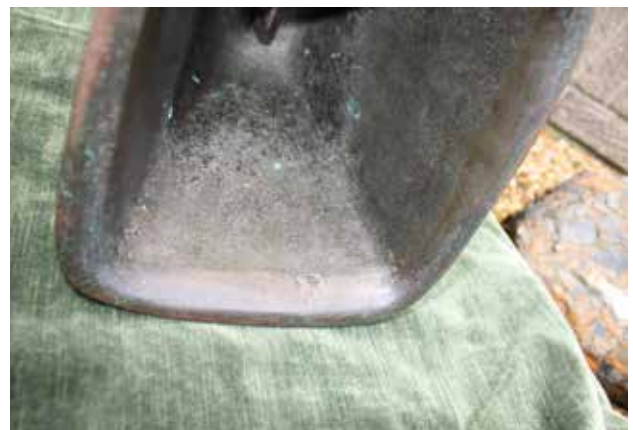
Figure 7.26 Handle of the bell, showing the flaw filled with lead, and attachment method
