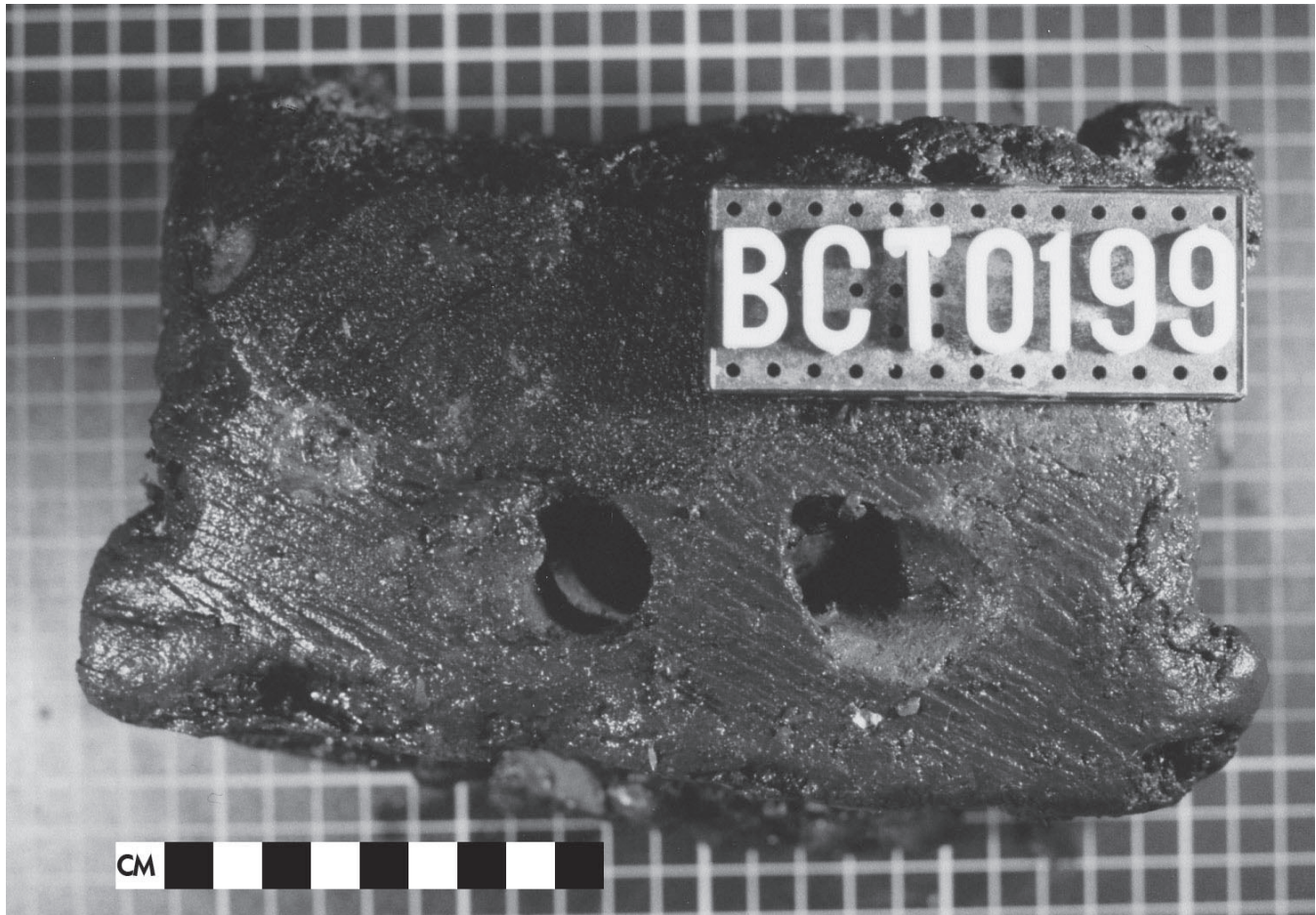
Figure 13.1 Image showing piddock damage to organics such as wood. Piddock damage has been seen to penetrate beyond a metre into the seabed (Garry Momber)
