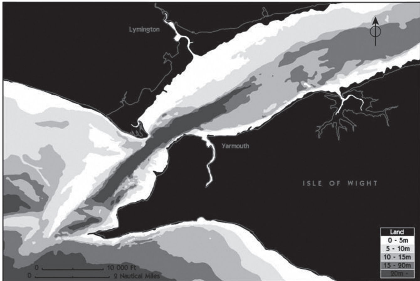
Figure 10.6 Bathymetric data from the Western Solent. The deep off Hurst Spit drops to almost -60\text{m OD} and gets shallower to the north-east and south-west. The shades of white and grey represent contours below Chart Datum (Drawing by Rory Smith with detail from Admiralty Chart 2040, 1991)
