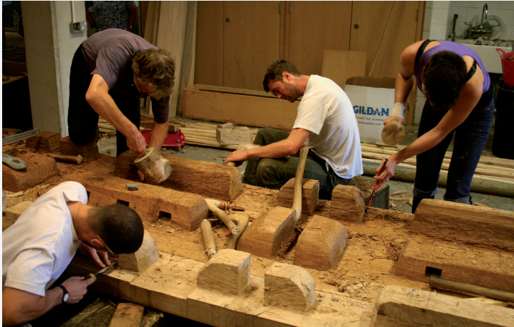
Figure 3.9 Work underway as part of an AHRC-funded project to construct a full-scale sewn-plank boat in the style of the Ferriby Bronze Age finds. © (left) Robert Van de Noort; © (right) National Maritime Museum Cornwall
