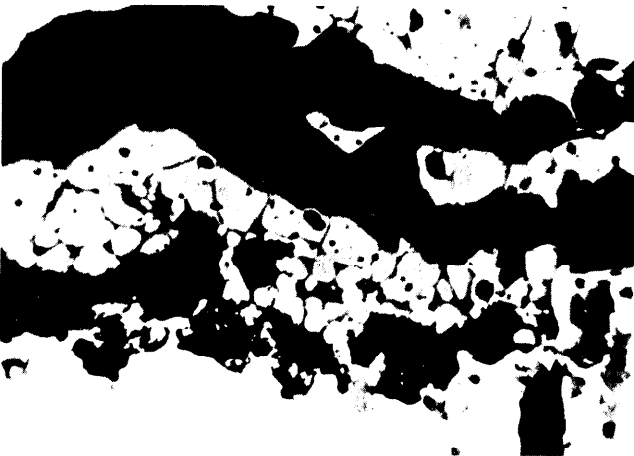
Fig 41 Scale formed by the oxidation of wrought iron at 1050°C (×125)
