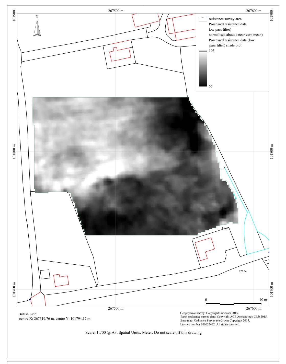
Figure 9: shade plot of processed earth-resistance data (low pass filter)
