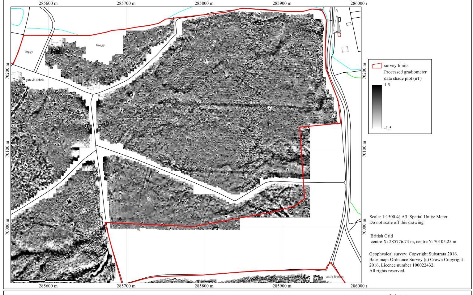
Figure 14: processed gradiometer data: area B; plots 5, 6 and 8
