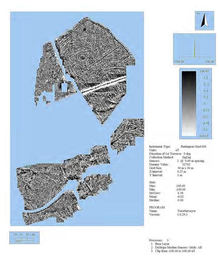
Figure 23: shade plot of minimally processed gradiometer data: area D; plots 17, 18, 21 to 24
