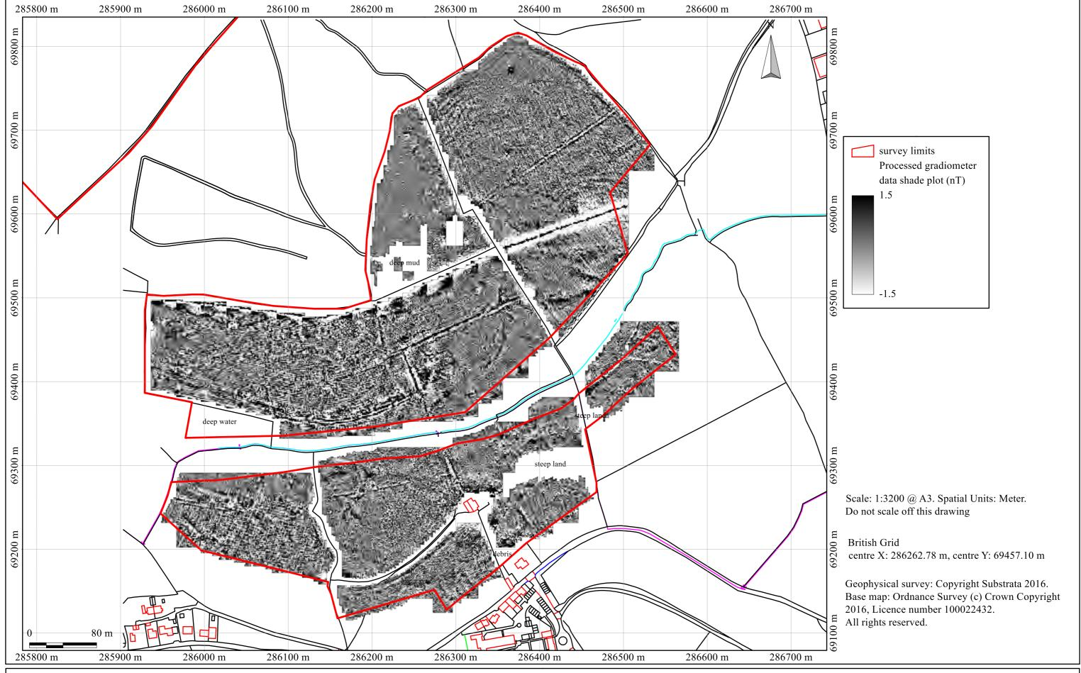
Figure 12: processed gradiometer data, area D
