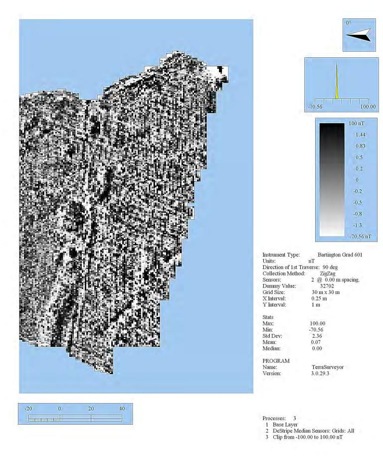
Figure 24: shade plot of minimally processed gradiometer data: area D; plot 25
