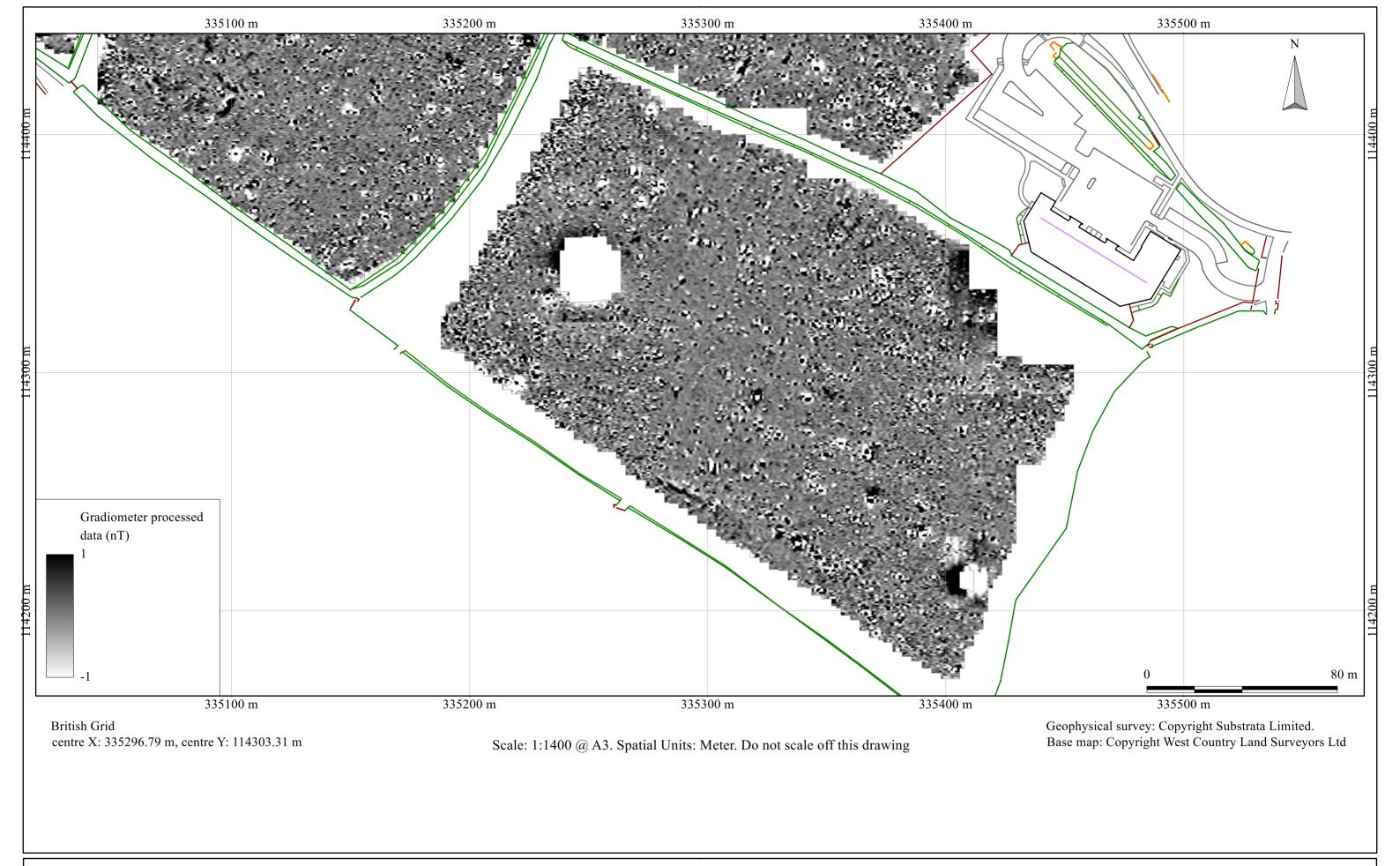
Figure 13: shade plot of processed data, field 5
