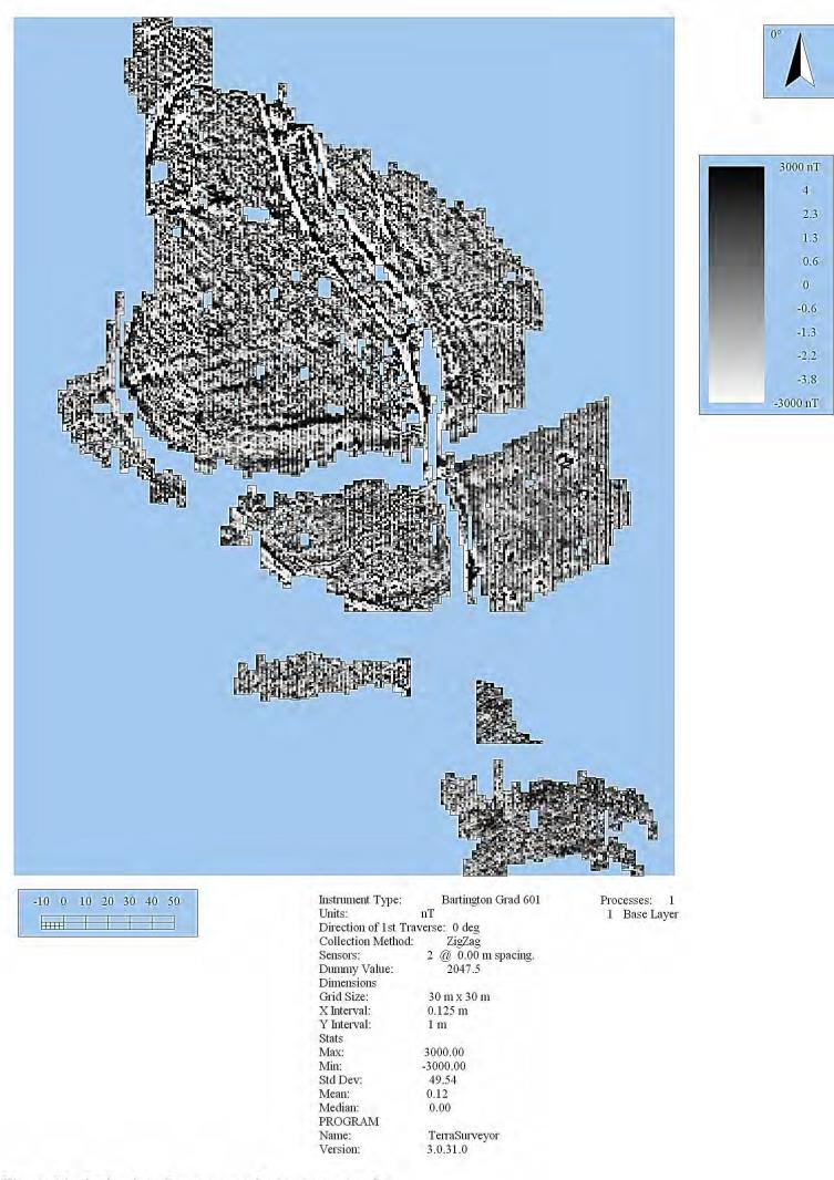
Figure 14: shade plot of unprocessed magnetometer data
