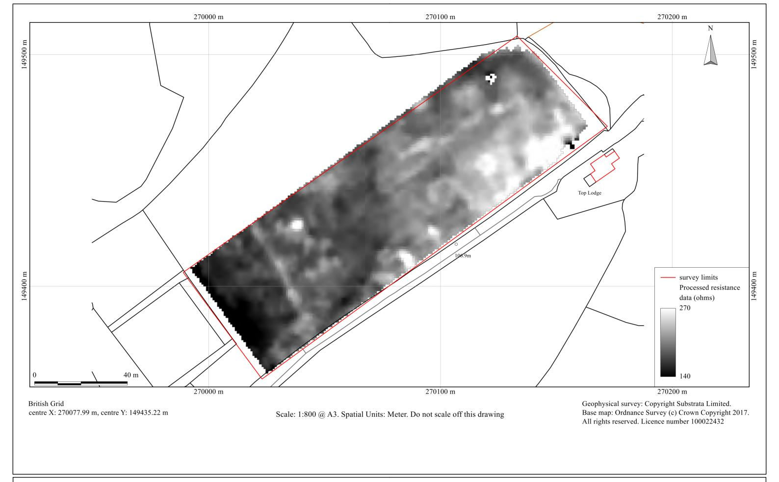
Figure 7: shade plot of processed resistance data
