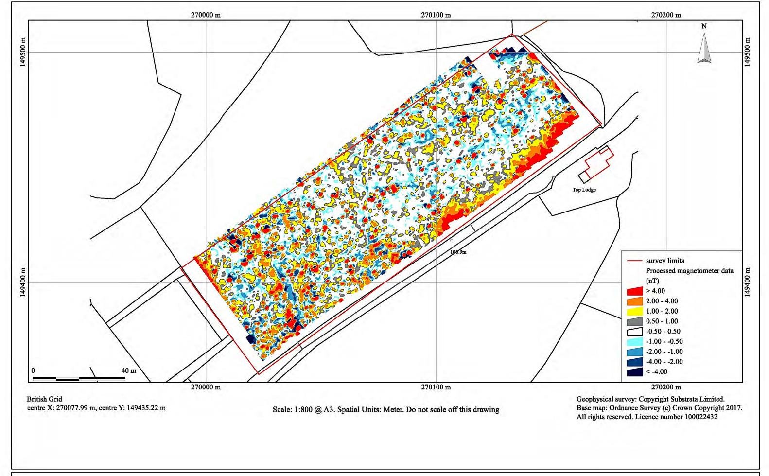
Figure 6: contour plot of processed magnetometer data
