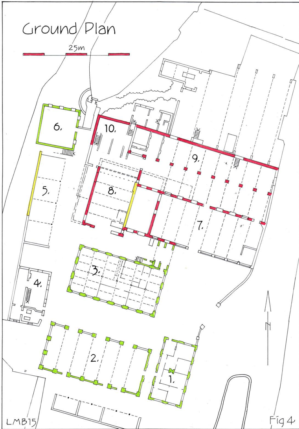
Fig. 4; ground floor plan, yellow is for masonry, red is 1856 fabric and green 1864 fabric
