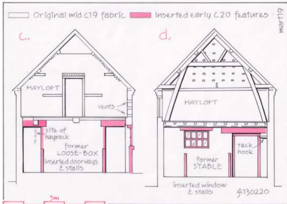
Fig 8; The North-East Range; sections to south-east.
