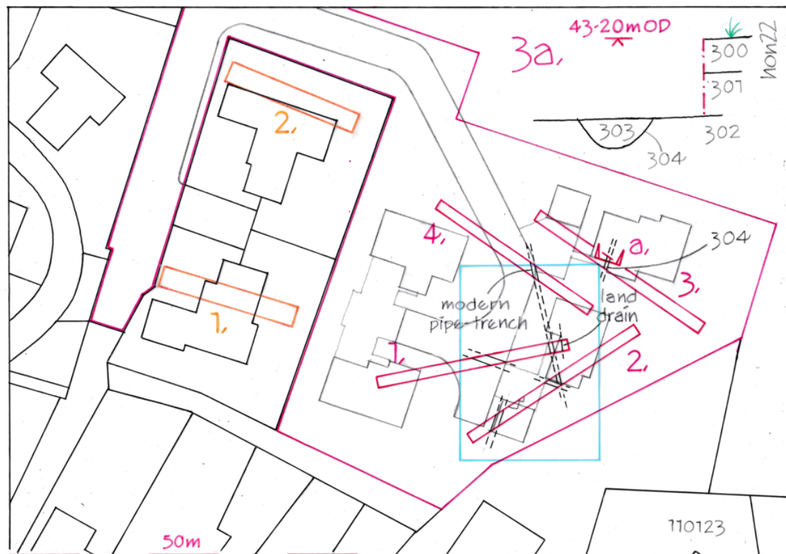
Fig. 3: site plan with trench locations, also showing main archaeological features and a detail of [304]. The blue inset (Fig. 4) details the features in this area. The orange trenches are from the 2015 evaluation. The proposed development including new access road, house plots and their associated driveways are in grey.
