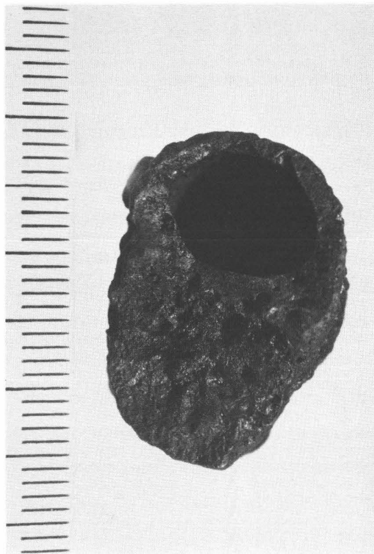
Fig. 12. End view of slag 'pipe' at Bexhill—enlarged, showing heavier accumulation of slag on lower side.
