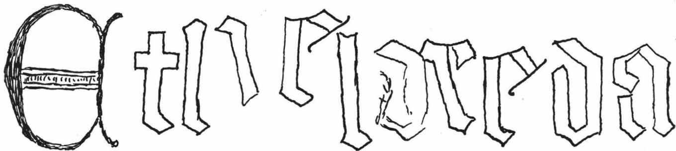
48. Flaw on the 4th bell at S. Nicholas, Feltwell, Norfolk, a Norwich bell of the 15th century, showing how the wax letters on the clay model of the bell were displaced by the superposition of the clay to form the cope.
