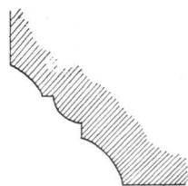
MAULING ON BOTTOM OF BEAM AT WEST END OF HALL.
