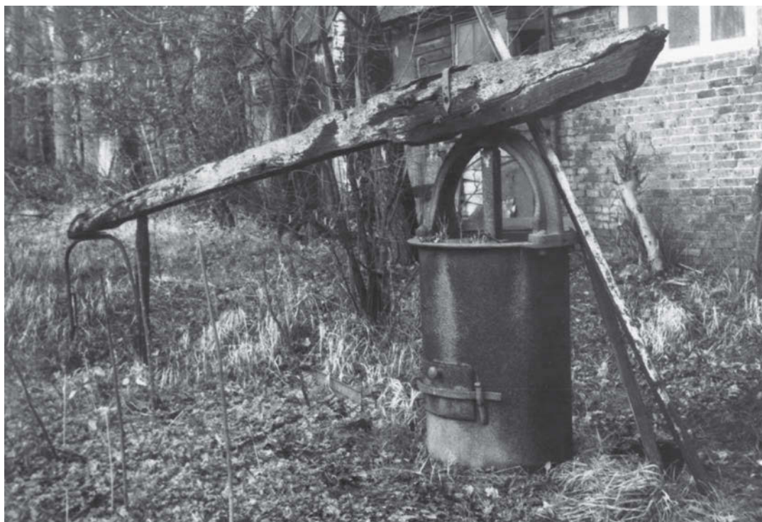
Fig. 8. Photograph of the horse-driven pug-mill, showing the horse harnessing at the end of the wooden arm; taken at the East Grinstead Pottery works (courtesy of East Grinstead Museum Collection).
