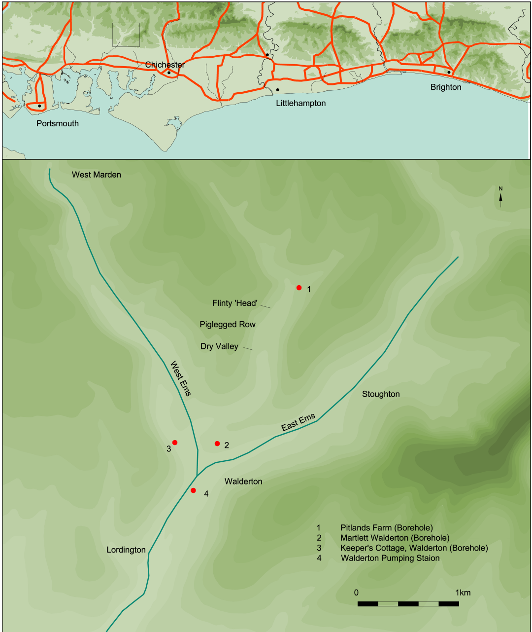
Fig. 12. The positions of boreholes and the pumping station at Walderton Bridge, West Sussex.
