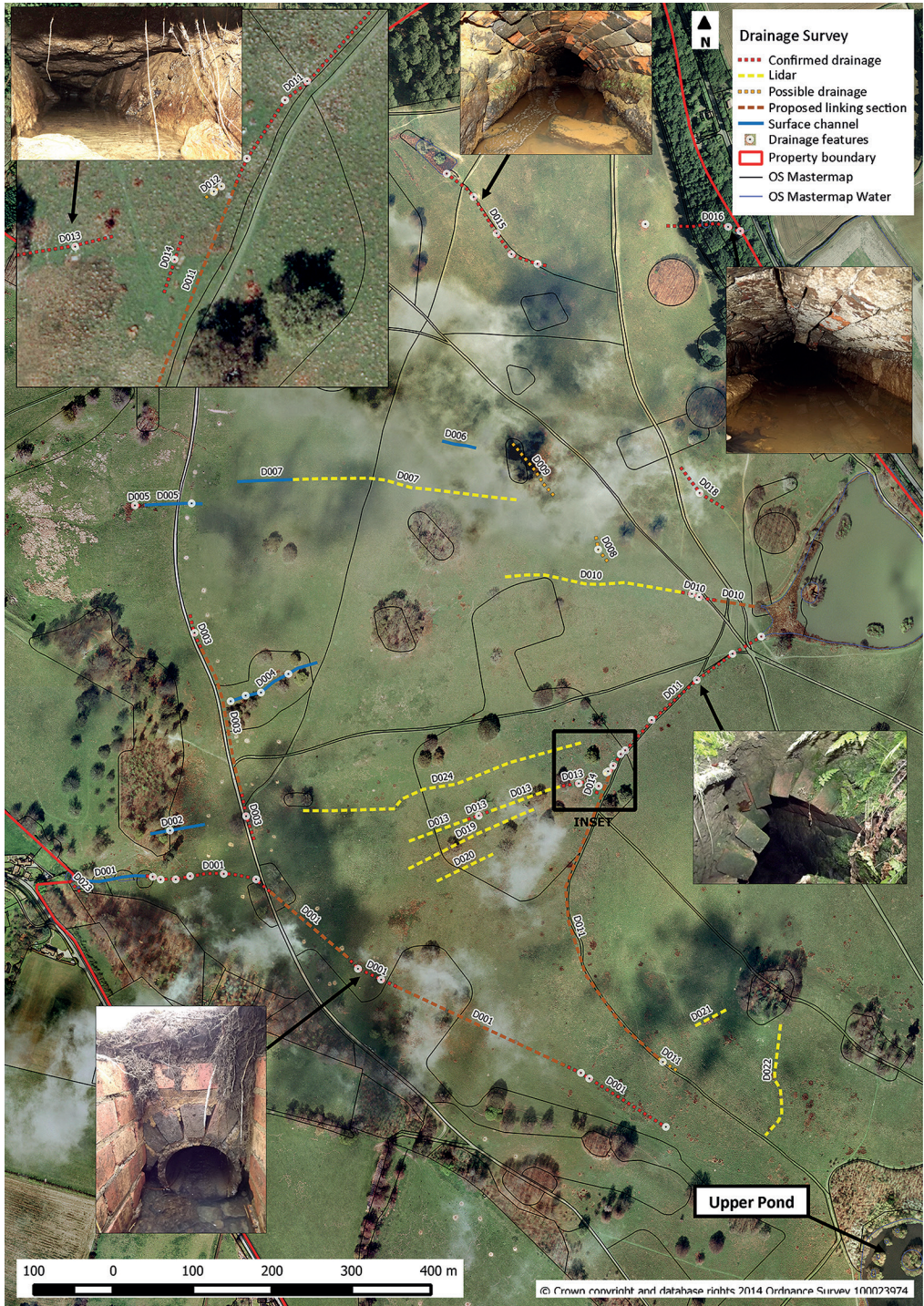
Fig. 19. Various forms of drainage in the north of Petworth Park, mapped through field survey and analysis of LiDAR data.
