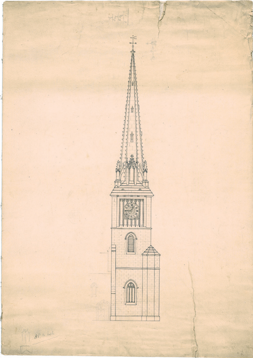
Fig. 13: Petworth, St Mary: south elevation of tower, spire and stair turret, undated and unattributed (WSRO, Par 149/4/2; courtesy West Sussex Record Office)
