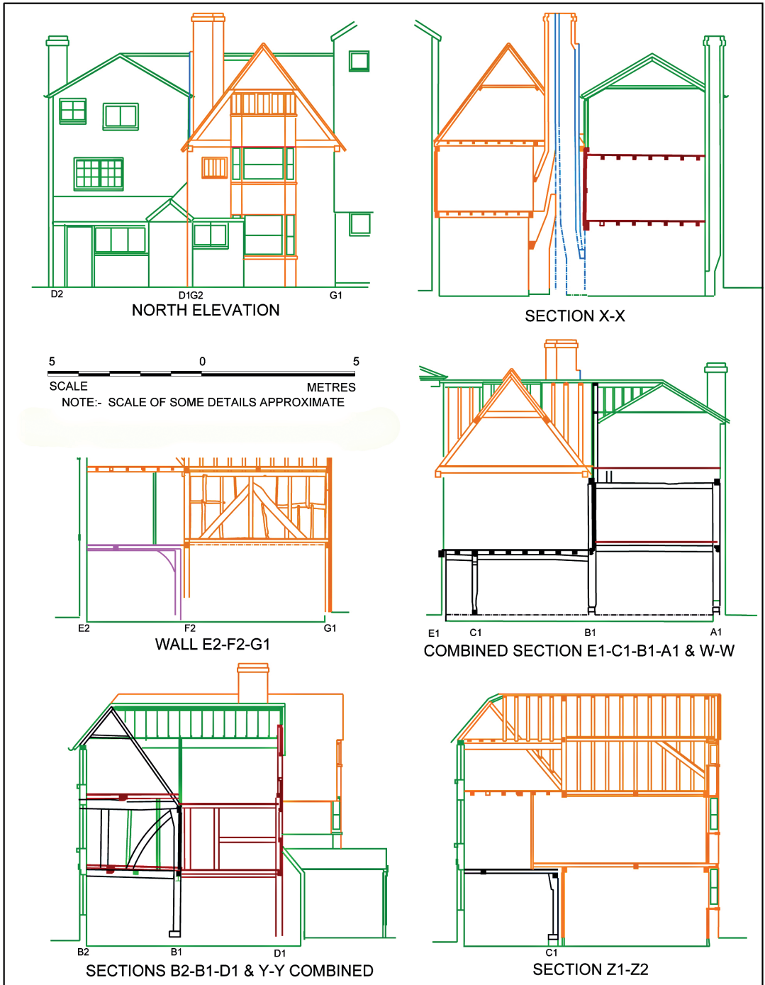
Fig. 3B. Interpretation of the architect's drawings made prior to renovation in 1987, B: north elevation and sections.
