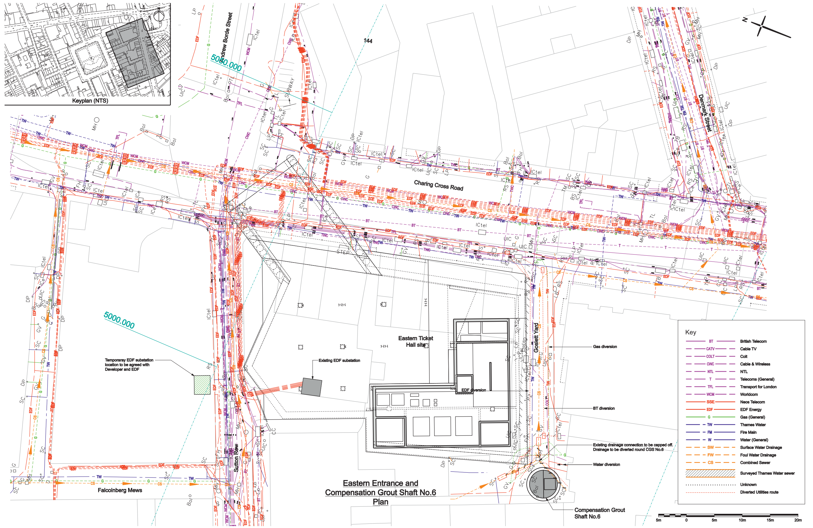
Fig 3 Tottenham Court Road Station eastern entrance, compensation grout shaft no 6 and utility diversions (Crossrail drawing P20700-C1M08-U00-D-00012)
