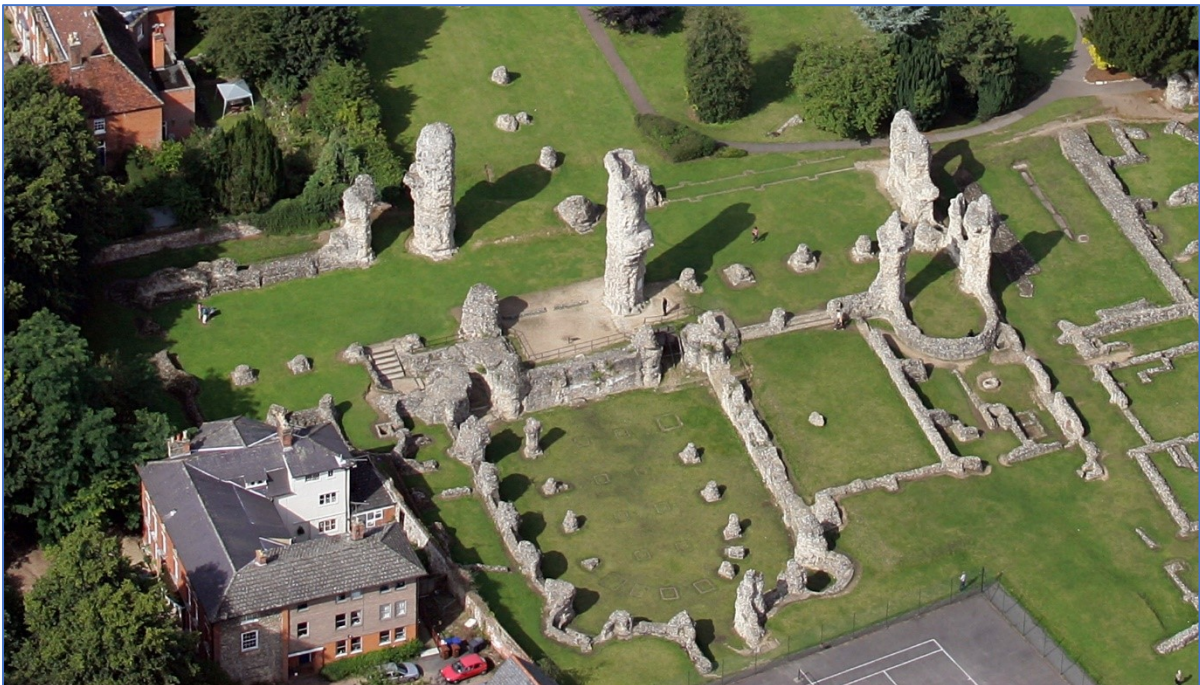
Figure 100: Aerial view of the crossing, looking north-west, showing the pier footings in the crypt, the surviving elements of the crossing piers and the piers of the eastern aisles of the north and south transepts. (© Mike Page, reproduced with permission)
