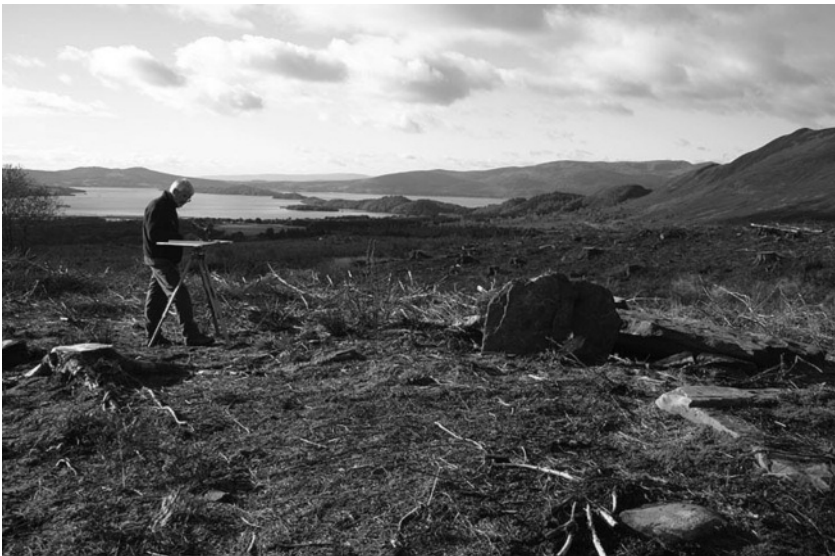
Figure 1. Ian Parker (RCAHMS) undertaking a measured survey of the chambered cairn by plane table and alidade. One of the upright slabs is visible centre right, alongside the two capstones.
