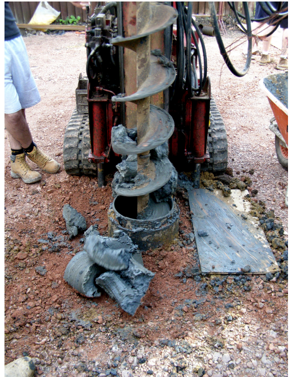
2. The drill in operation, bringing up ?riverine alluvium, context (102)
