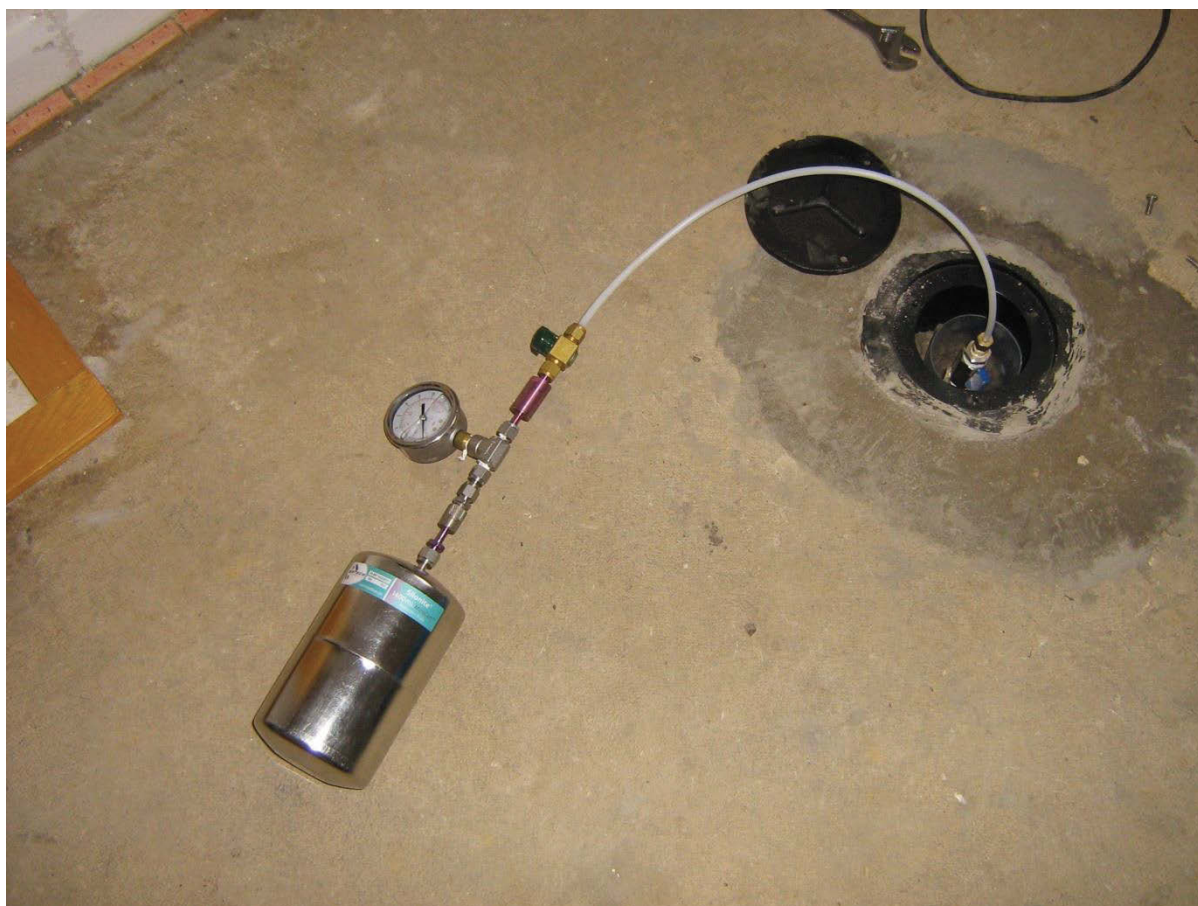
Figure 9 Gas Sampling from a Borehole using a Vacuum Canister
