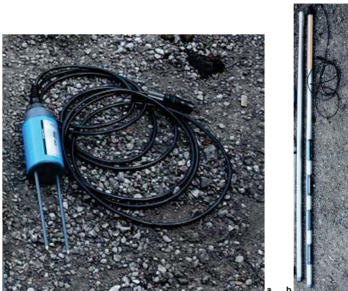
Figure 18 a) Trime Pico 64/160mm probe; b) Pico T3P Profile Probe
