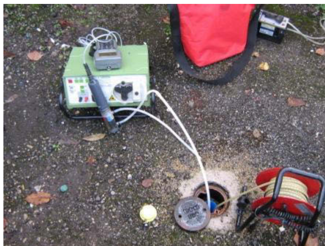
Figure 10 Dipwell with monitoring of water quality and groundwater level in progress
