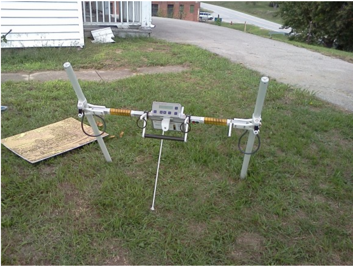
It's not a spaceship, it's a magnetometer.
