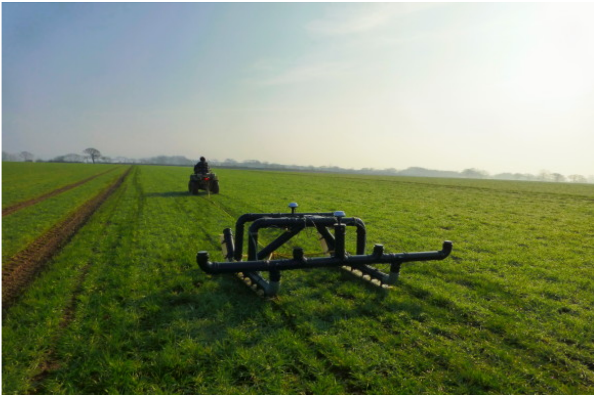
The towed caesium vapour, GPS guided magnetometer sled
