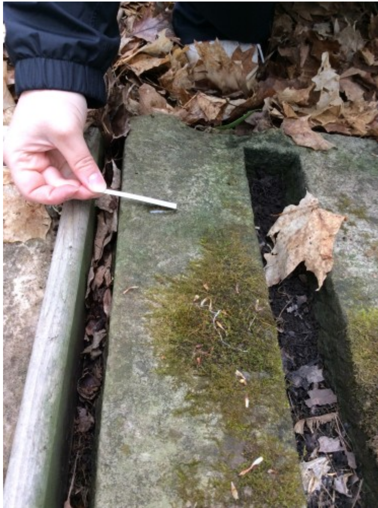
We're testing the pH level of a gravestone to assist with a condition assessment.
