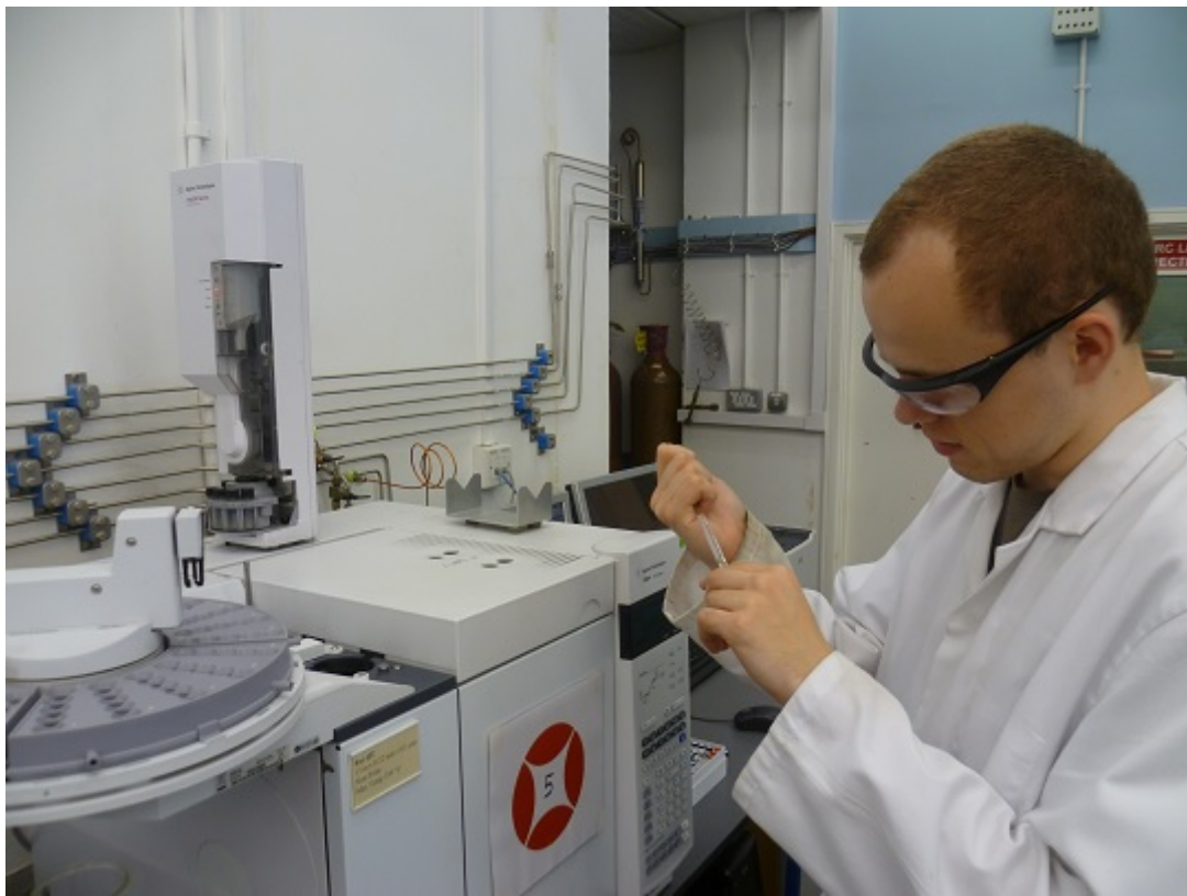
David about to inject part of a sample into a gas chromatograph
