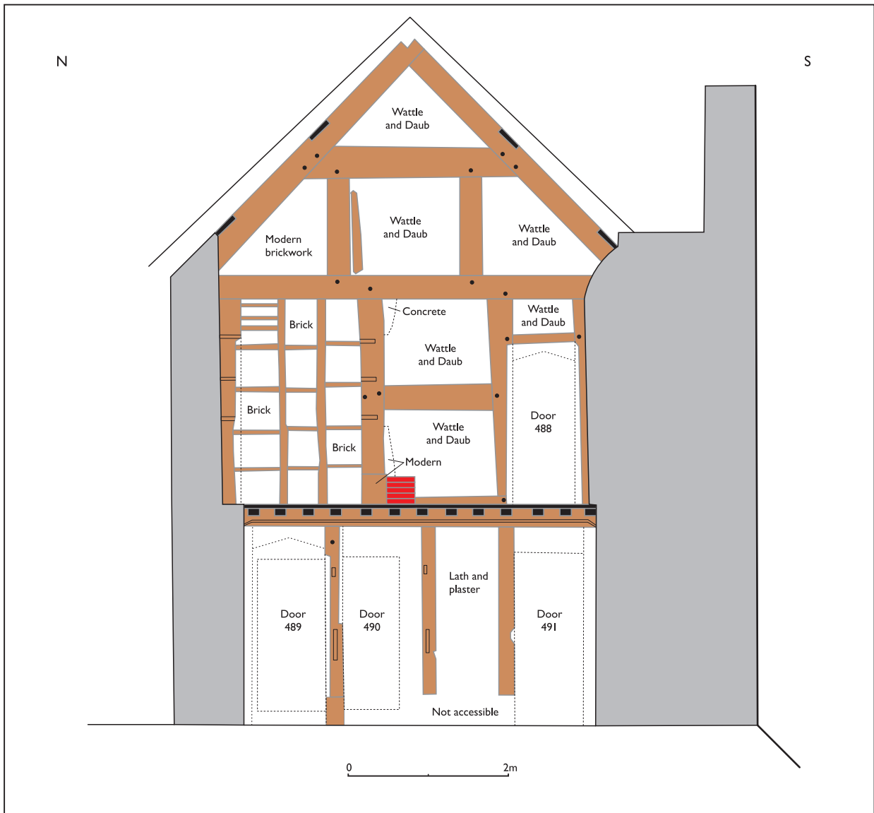
Figure 13.6: West facing elevation of Truss 4 in rooms 26 and 118 in Castle House. After record drawings by Keystone and James Brigers (Thorp and Cox 2013, Figs 25, 63 and 65).
